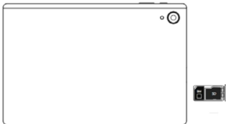
Following the instructions illustrated in above picture, you can insert the Nano SIM card into the SIM tray with gold contacts facing down, or remove the Nano SIM card from the sim tray.
