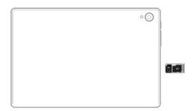
Following the instructions illustrated in above picture, you can insert the Nano SIM card into the SIM tray with gold contacts facing down, or remove the Nano SIM card from the sim tray.
